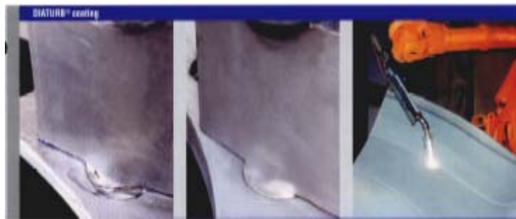
Fig 20 Coating on Francis components
