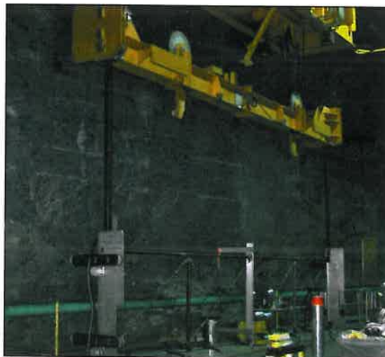
Current meter trolley attached to a gantry crane.
